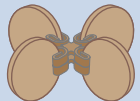
Extra Strength By doubling connectors you can strengthen any connection. (This shows two 4-way connectors.)
