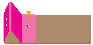
Insert the ends of the test tube holder into the pair of holes on the cardboard, and then move it down, as shown.
