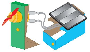
Place the solar cell under a bright light bulb so that the propeller rotates.
